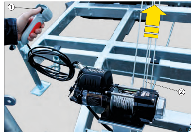
Fig. 11 Controlling cable winch
