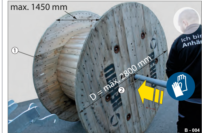
Fig. 6 Inserting transport shaft
