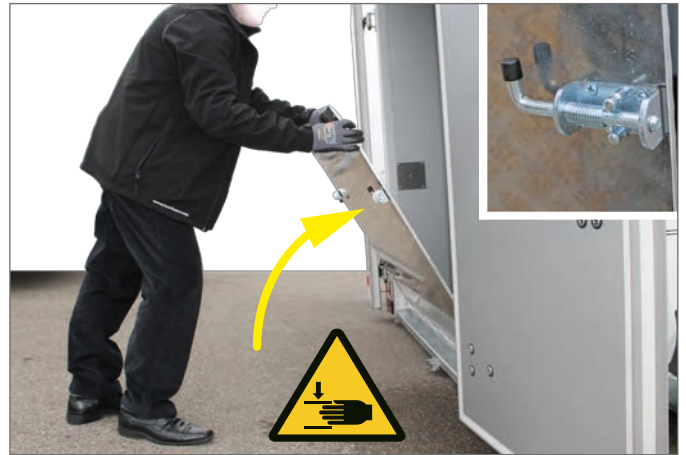
Folding up the ramp front edge
