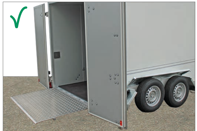
Ramp front edge folded down
