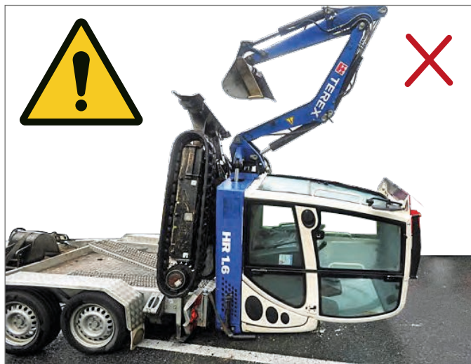
Example of accident (mini-excavator was not tied down)
