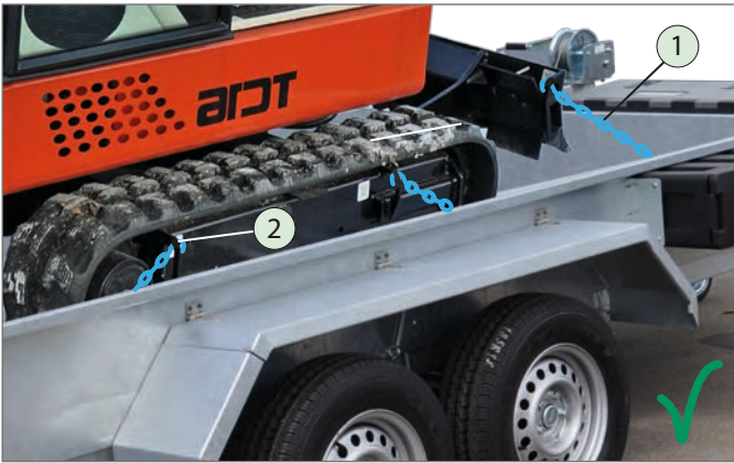
Example of "force-fitting load securing" / mini excavator
