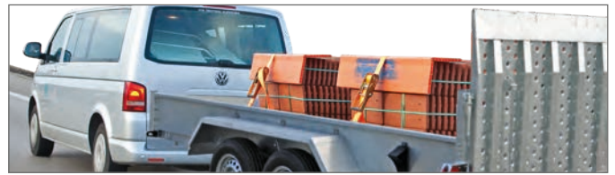
Example of "force-fitting load securing"
