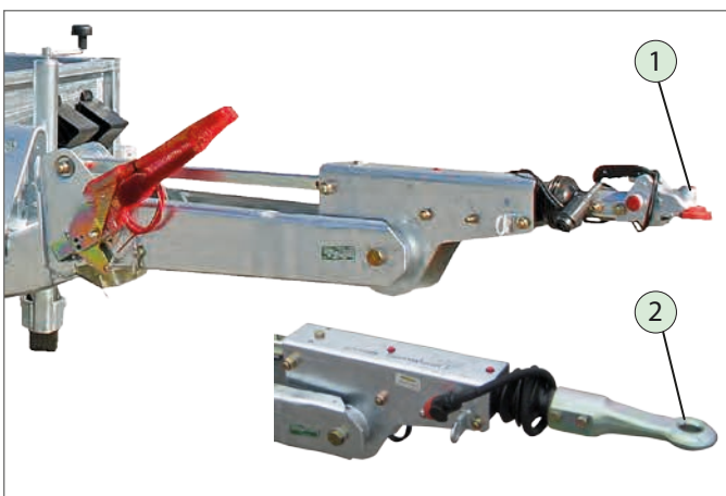
SENKO - HV-shaped drawbar (ball coupling)
