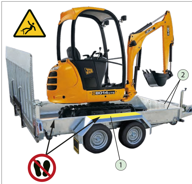
Stepping onto the steel mudguards
