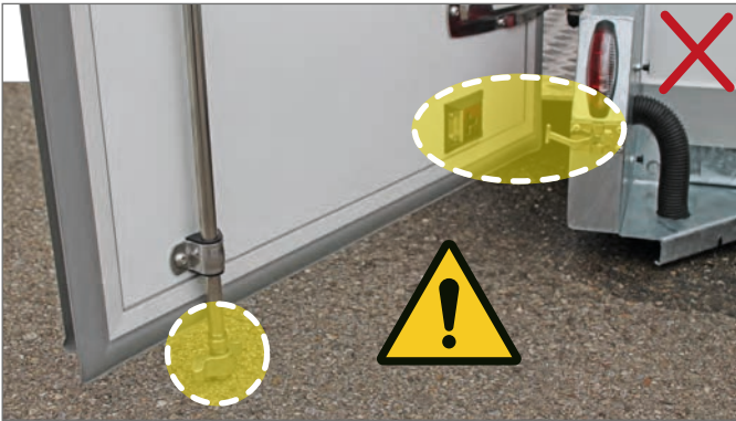
Negative example - unsecured door stop
