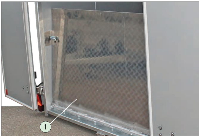
Ramp front edge secured
