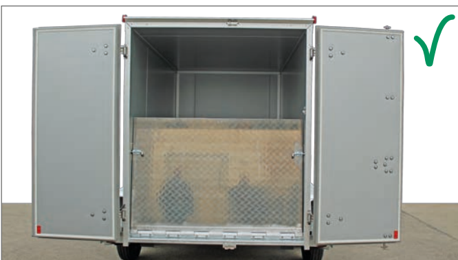
Double wing door folded open and secured
