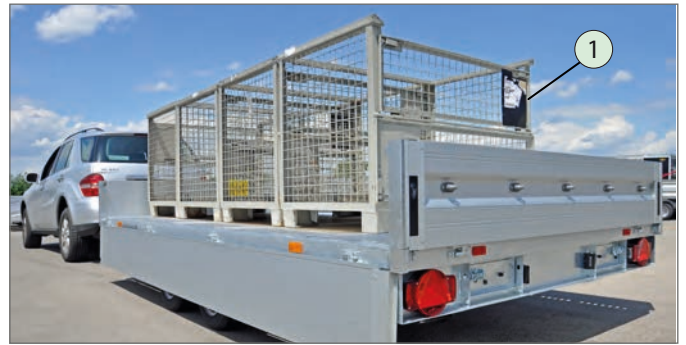
Example of "form-fitting load securing"
