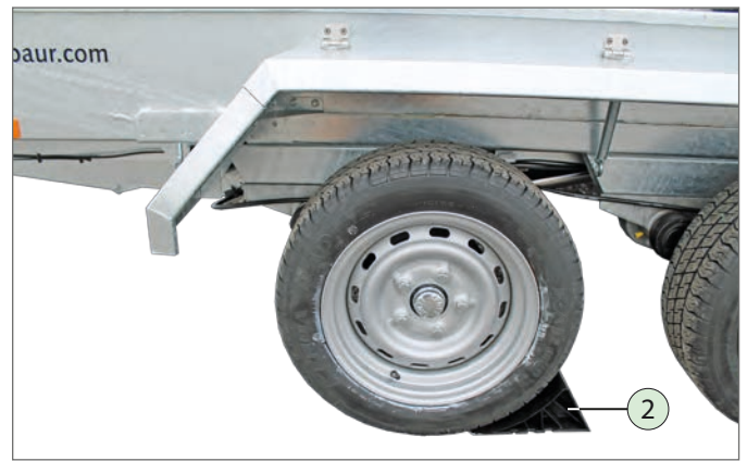
Wheel chock on rigid axle, front
