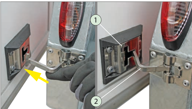
Securing the double wing door with the door stop
