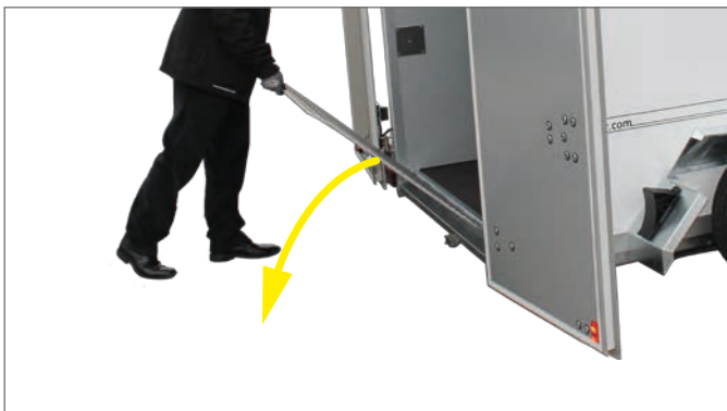
Fold down the ramp front edge
