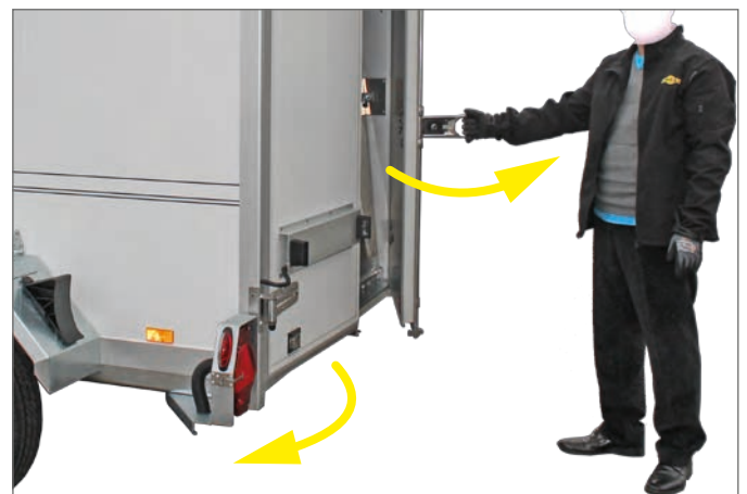
Folding open the double wing door
