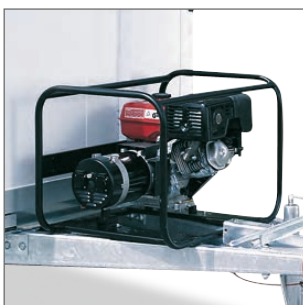
Power generator on the drawbar
