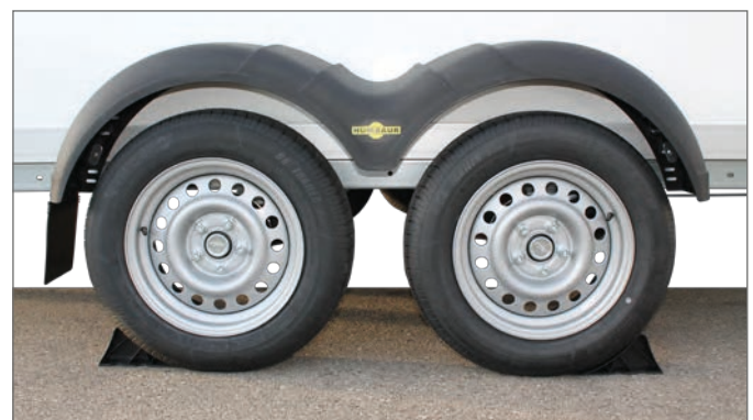
Placing the wheel chocks, tandem
