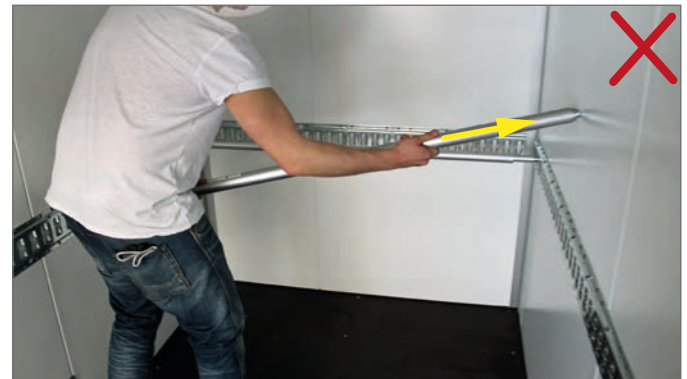
Damaging the inner wall
