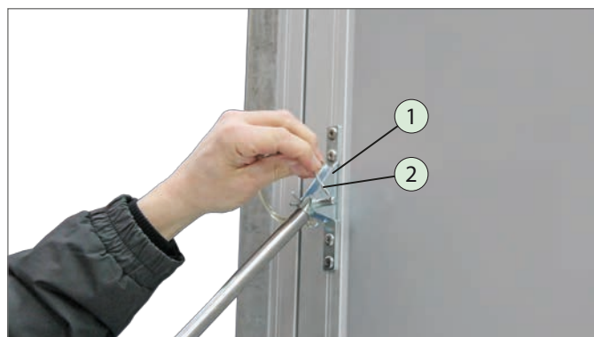
Securing the retainer
