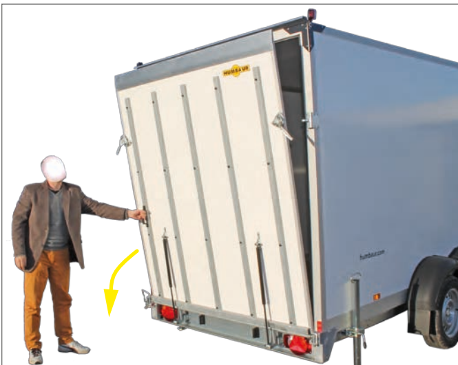
Lower ramp wall
