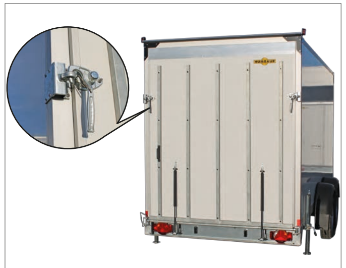
Angle lever lock closed, secured
