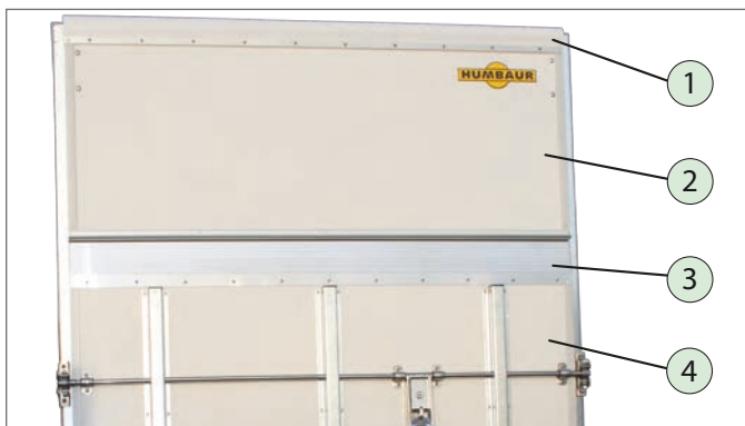
Ramp wall with top flap closed
