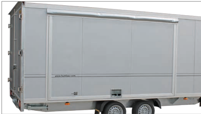
Sales hatch with drive-rod lock, driving position
