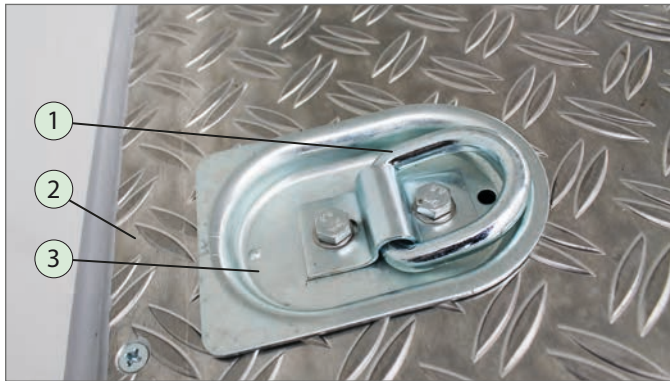
Tie-down ring recessed in tie-down groove (optional)
