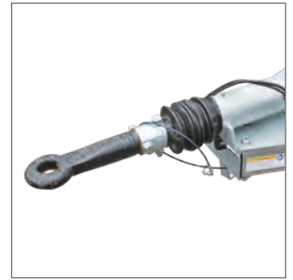
DIN towing eye for drawbar
