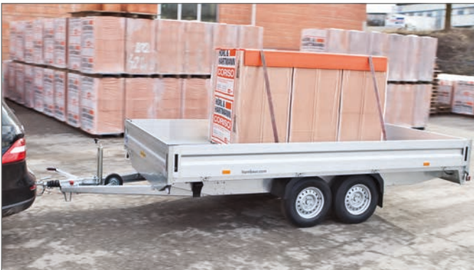
Secured with tie-down
