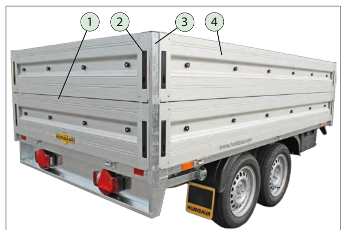
Side wall extension inserted
