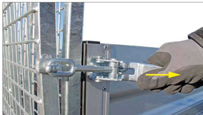
Securing the grid ramp wall
