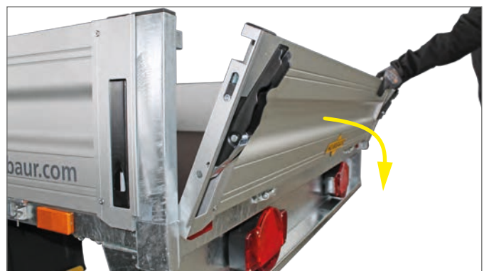
Folding down the rear drop side
