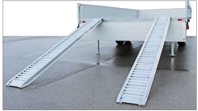
Drive-up ramps positioned
