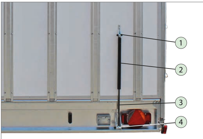
Gas strut of ramp wall
