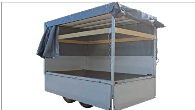
Sliding tarpaulin opened + drop side folded down
