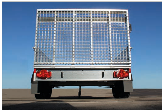
Grid ramp wall secured (driving position)
