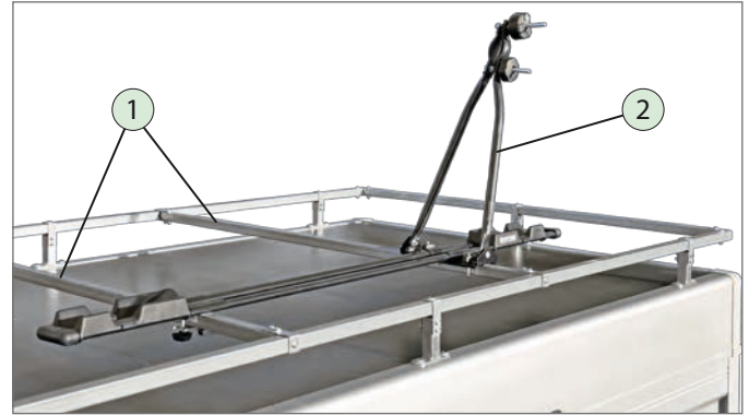
Bicycle stand attached to lateral crossbar
