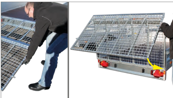
Grid ramp wall folded up
