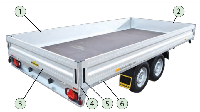
Drop sides and stanchions fitted
