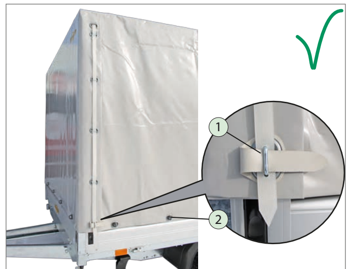
Tarpaulin cover closed / secured
