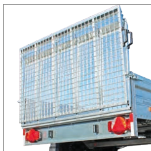
Grid ramp wall
