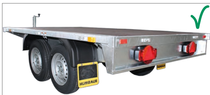
Driving as flat-bed (drop sides/stanchions removed)
