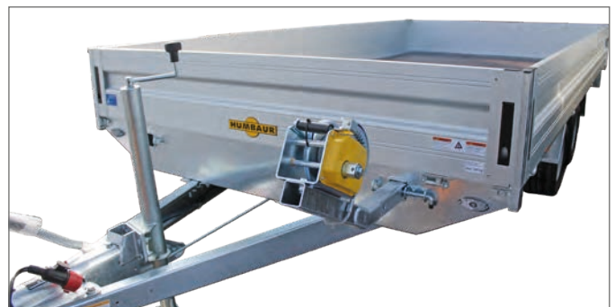
HN with cable winch frame, front view
