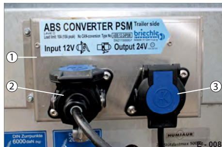
Fig. 13 ABS voltage transformer
