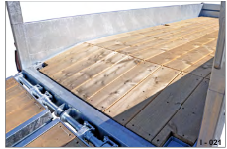
Fig. 21 Wooden planks (spruce, 40 mm)
