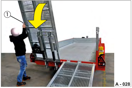
Fig. 30 Lowering the ramp
