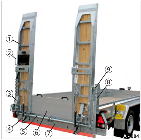
Fig. 13 HS with steel ramps, with gas pressure spring support
