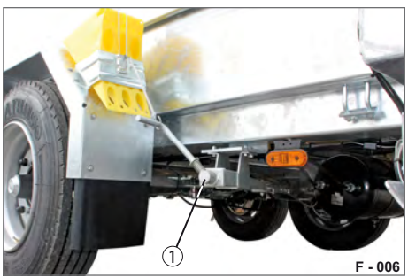
Fig. 6 Controls - rear side (HS 10xx) 1 Spindle parking brake
