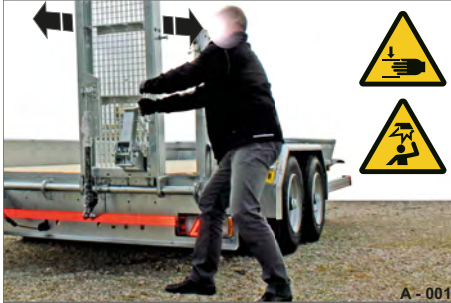
Fig. 10 Operating drive-up ramps
