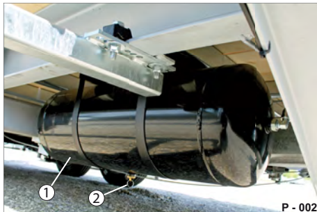
Fig. 51 Compressed air tank below frame
