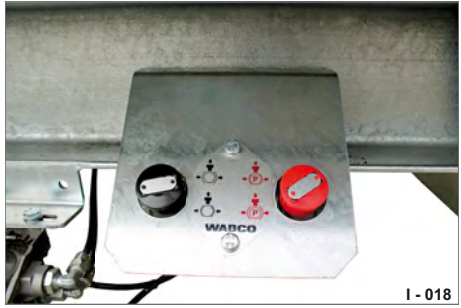
Fig. 18 Compressed air brake with spring-loaded cylinder
