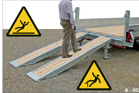
Fig. 11 Walking on drive-up ramps
