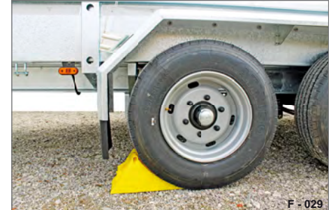
Fig. 55 Example: Wheel chocks in place
