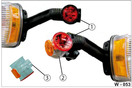
Fig. 53 Removing the rubber arm 1 Rubber arm covering 2 Lamp 3 Screw fitting
