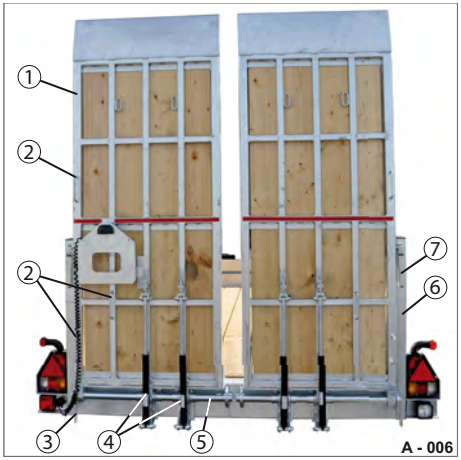
Fig. 15 HS with wide steel ramps, with gas pressure spring support
