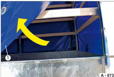
Fig. 77 Opening curtain section
