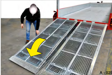
Fig. 31 Setting the ramp down
