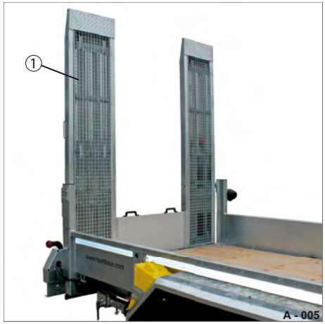
Fig. 14 HS with steel ramps, with gas pressure spring support
