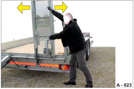
Fig. 25 Setting track width
