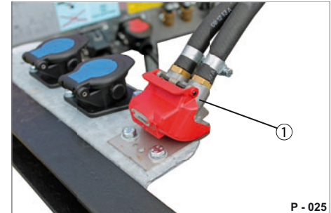
Fig. 12 Duo-Matic quick-release coupling system
