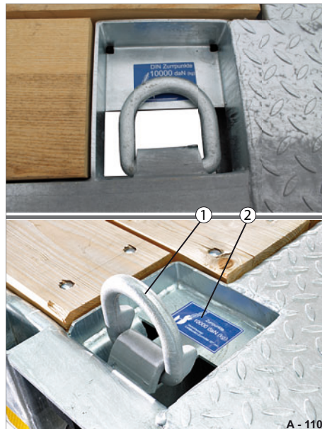
Fig. 127 Lashing point, up on loading platform: 10,000 daN (kg)
