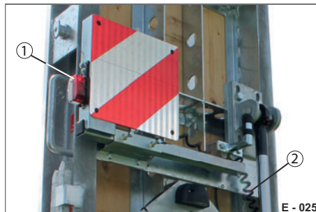
Fig. 19 Peripheral light on the warning panel, rear side on ramps
