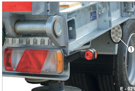
Fig. 16 Side position of the working lights
