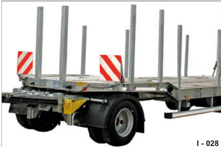
Fig. 21 Posts, can be inserted/removed
