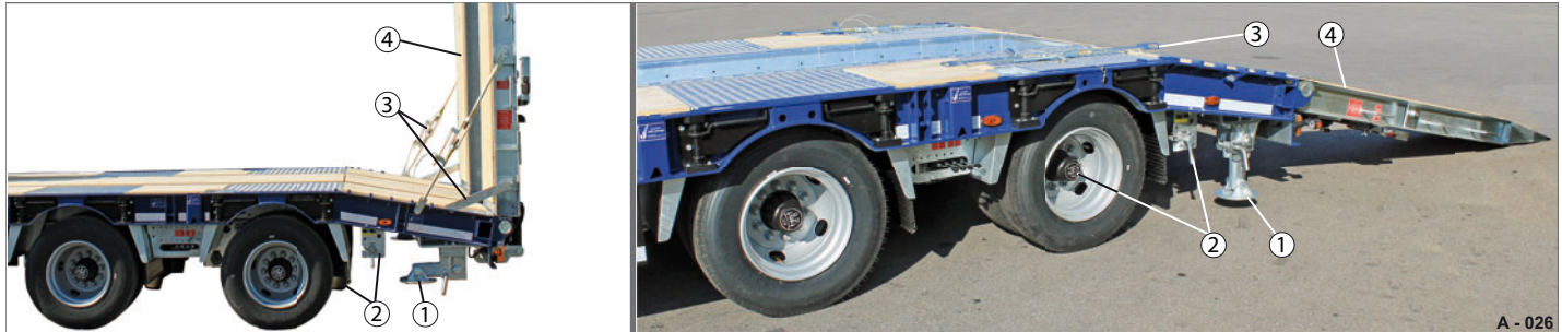
Fig. 27 Ramps are secured in drive position and ready for the loading/unloading process
