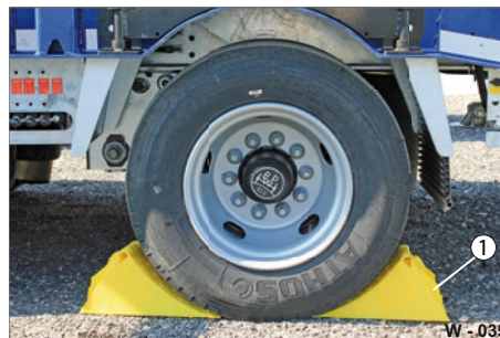
Fig. 35 Secure the vehicle
