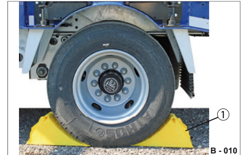
Fig. 15 Wheel chocks positioned
