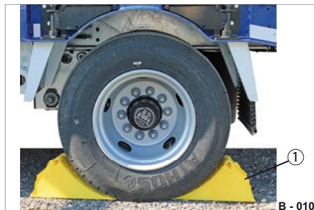
Fig. 44 Wheel chocks positioned
