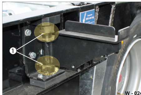
Fig. 23 Lubricating bearing points
