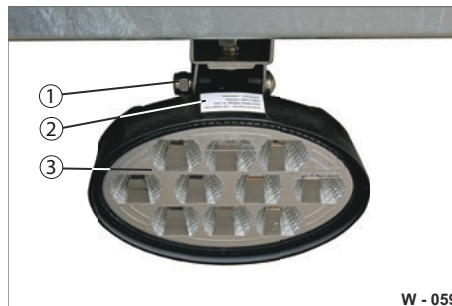
Fig. 59 Working light fixation
