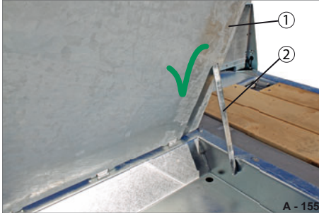
Fig. 73 Lid open, secured
