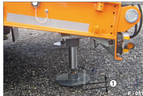
Fig. 61 Support props lowered, (position for loading/unloading) 1 Distance to ground (approx. 3-5 cm)
