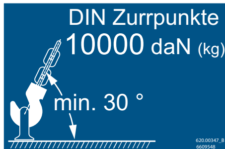
Fig. 124 Example: Label on lashing point
