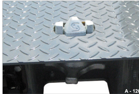
Fig. 142 Locked (container transport)
