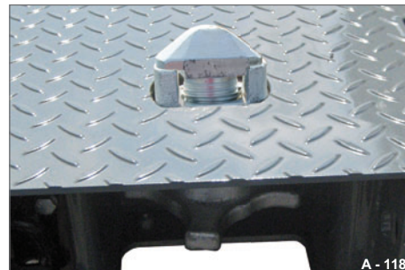
Fig. 140 Locking point in intake position
