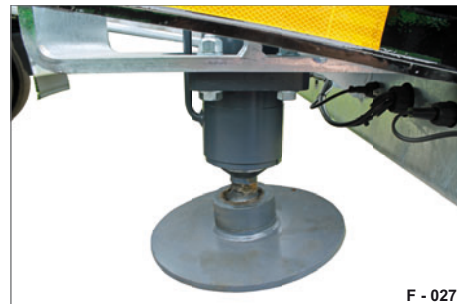
Fig. 60 Hydraulic support feet, folded up (drive position)
