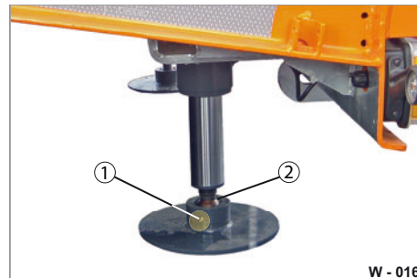
Fig. 12 Lubricating support props
