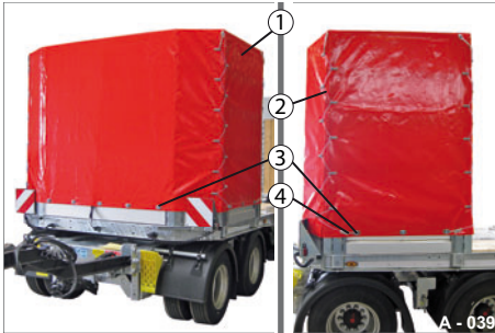
Fig. 43 Curtains/roof bow secured
