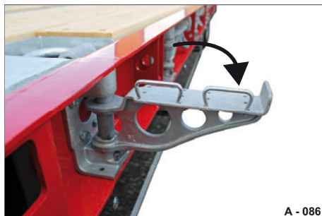
Fig. 77 Folding boom, folded out
