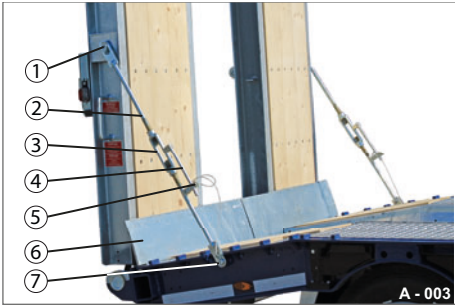
Fig. 3 Ramps secured with turnbuckle (with ramp cover plate)
