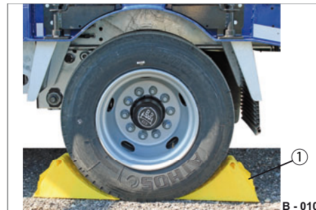
Fig. 98 Wheel chocks in place
