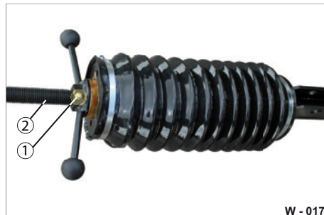
Fig. 13 Lubricating height setting
