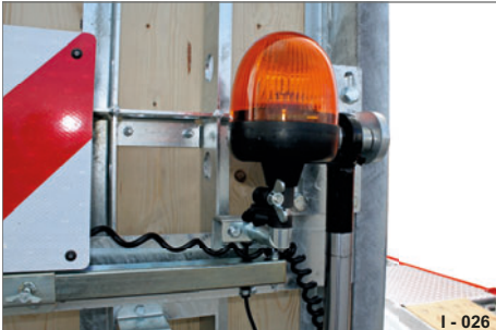
Fig. 19 Rotating light on rear
