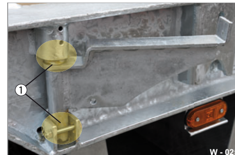
Fig. 24 Lubricating bearing points
