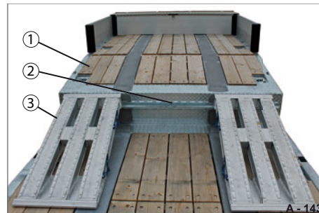
Fig. 152 High plateau can be driven over
