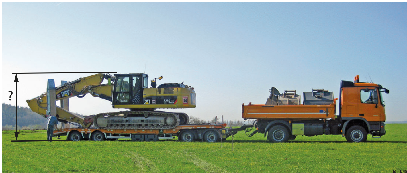
Fig. 58 Total height of the loaded flatbed
