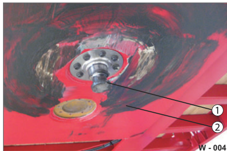
Fig. 4 Lubricating semi-trailer connection
