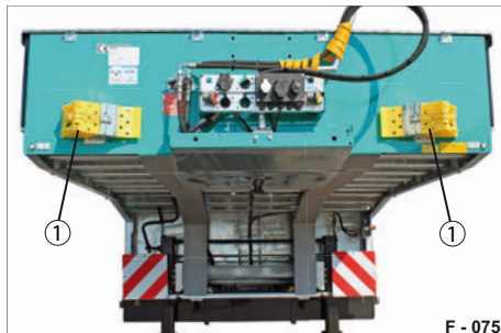
Fig. 103 Wheel chock, horizontal, in retaining brackets (steel plate)
