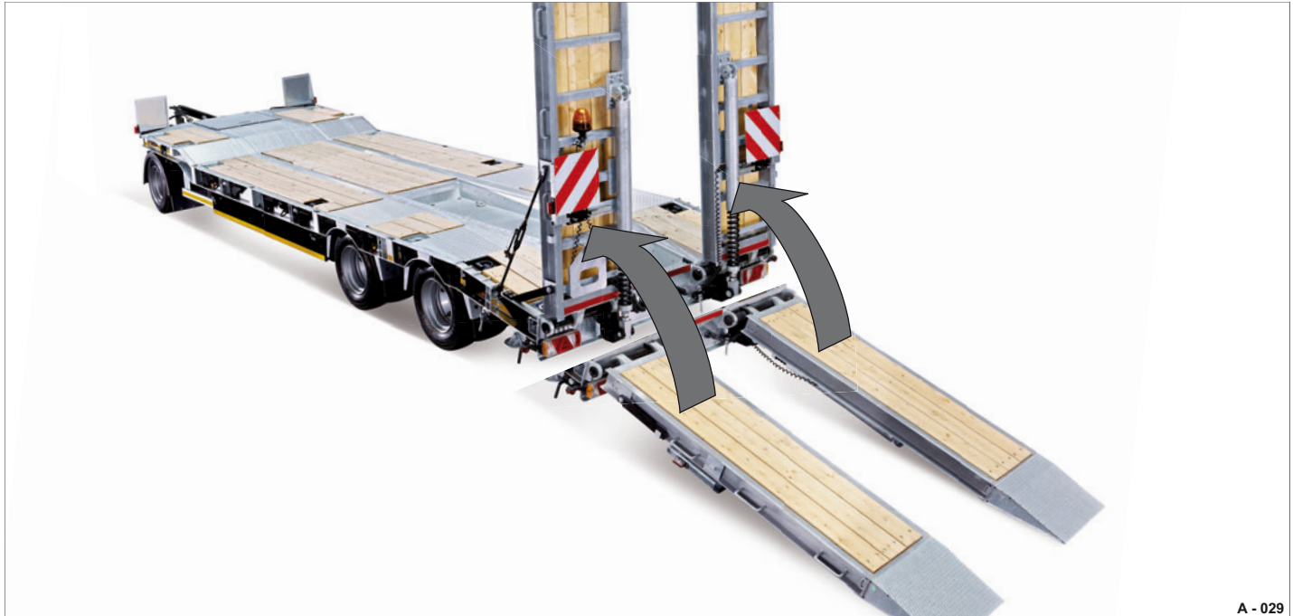
Fig. 30 Folding up ramps
