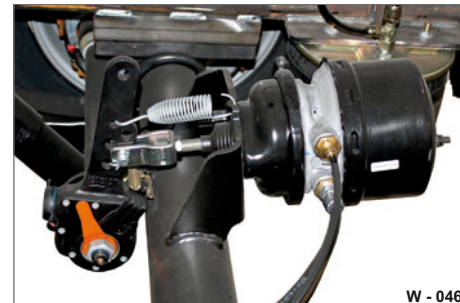
Fig. 45 Releasing spring tension
