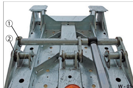
Fig. 21 Lubricating bearing points
