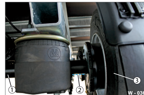
Fig. 36 Putting lifting device into position
