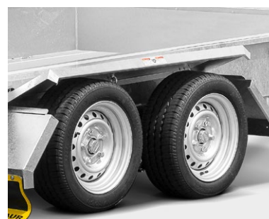
Steel mudguards, automatically opening and closing during the lowering process
