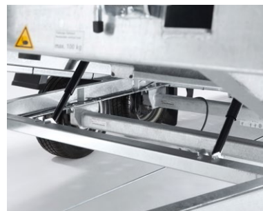
Bridge with special tilt bearing
