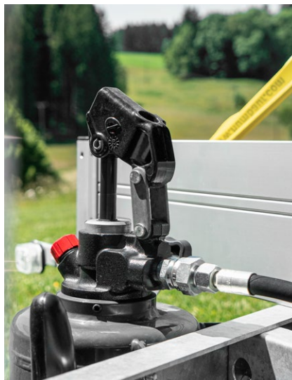
Hand pump with oil reservoir
