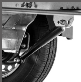
Wheel shock absorbers incl. 100 km/h confirmation
