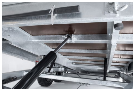
Special stability due to double hat profiles in transverse direction on the bridge
