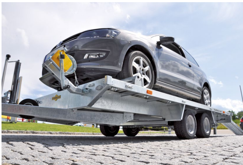
Stable base frame made of folded steel profiles
