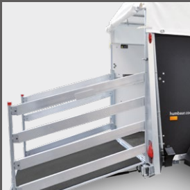
Drift fence on both sides on overrun flap
