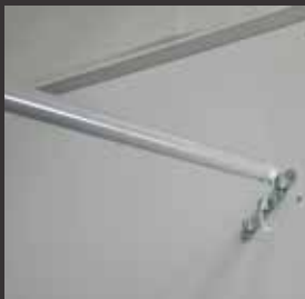
End-to-end box rod for transporting foals (standard on some models)
