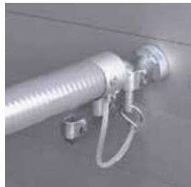
Three-way adjustable breast and breech bars
