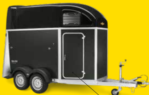
Large access door with three-point locking
