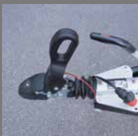
Safety coupling with track stabilisation
