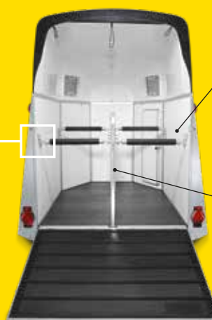
Three-way adjustable breast and breech bars
