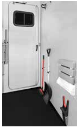
Saddle compartment with saddle holder and folding seat, boot jack, bridle holder, mirror, net, interior lighting, shovel and broom.
