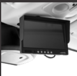
Monitor for the reversing camera in the cab
