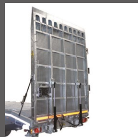
Hydraulic ramp wall with steel grating
