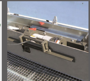
Winch on the loading area
