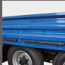
Forklift ram protection on the side
