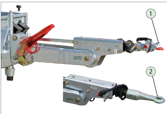
SENKO - HV-dissel (trekkogelkoppeling)
