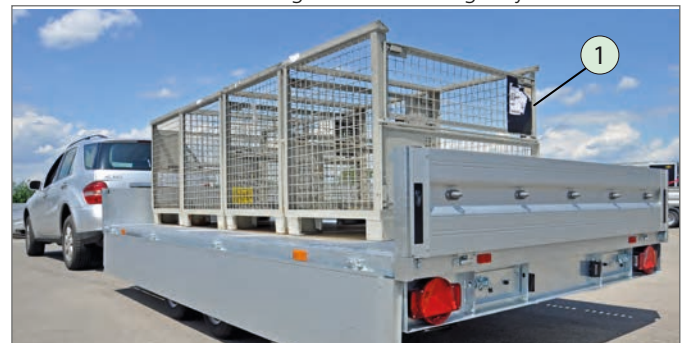
Example of "form-fitting load securing"
