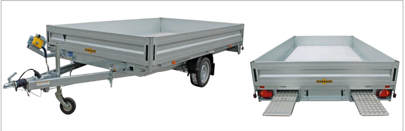
MTK single-axle trailer with 350 mm drop sides and loading ramps
