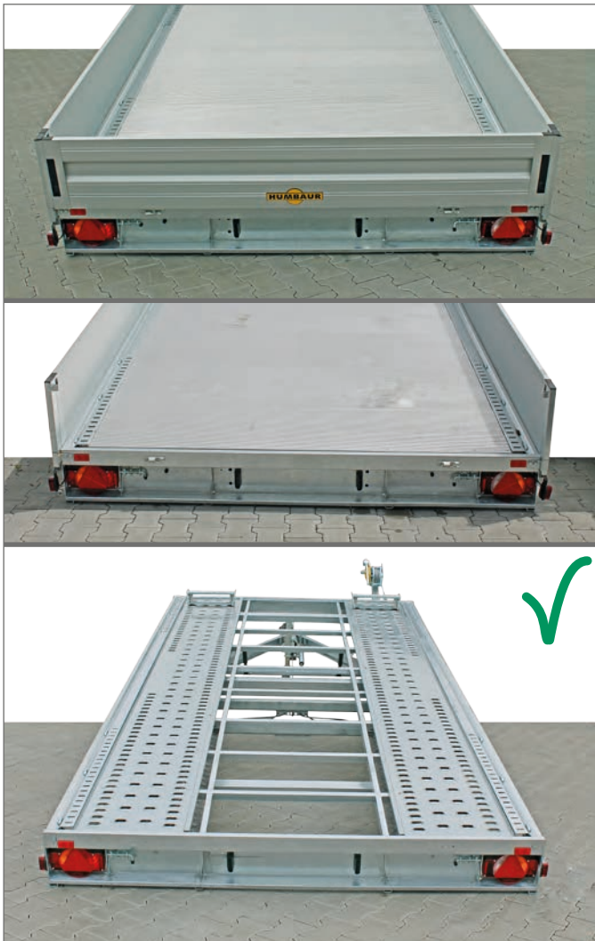
The underride protection is in complete contact with the ground.
