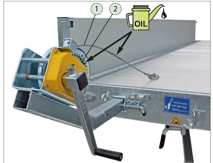
Testing / greasing the cable winch
