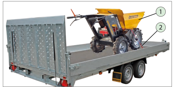
Example of "force-fitting load securing"
