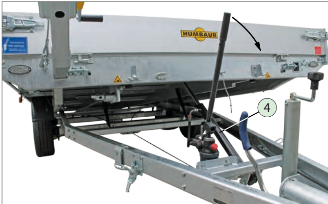
Cargo bed hydraulically folded down
