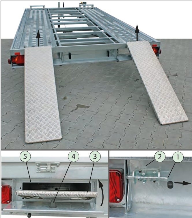
Loading ramps stowed away
