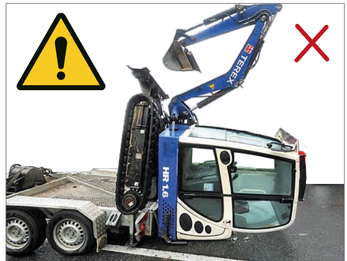
Example of accident (mini-excavator was not tied down)
