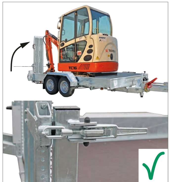
Loading ramp closed and locked
