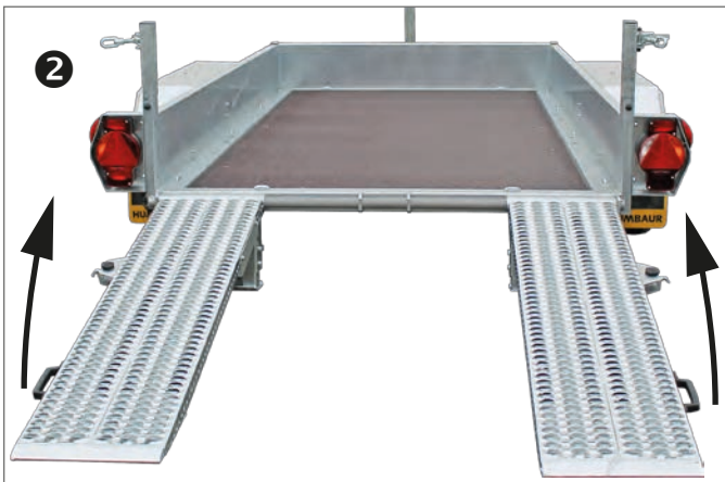
Closing the loading ramps
