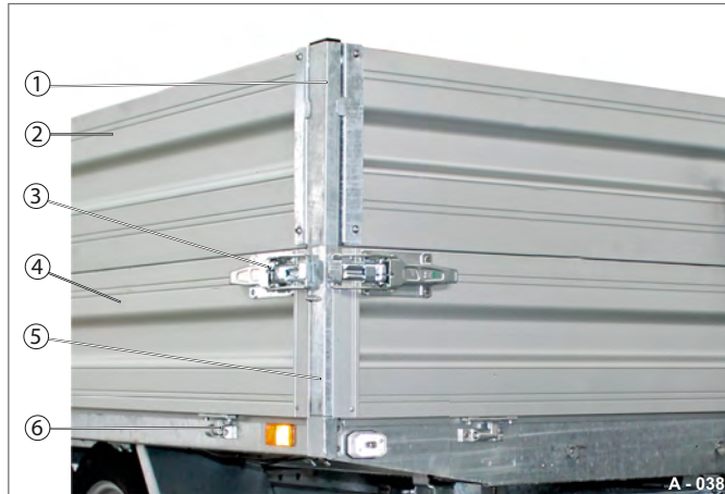
Fig. 29 Side wall extension fitted
