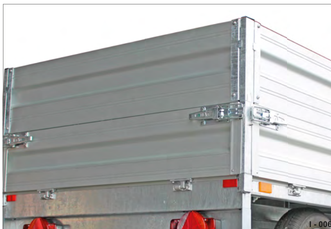
Fig. 6 Attached to stanchions
