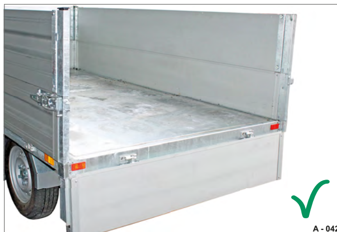
Fig. 33 Side wall extension removed
