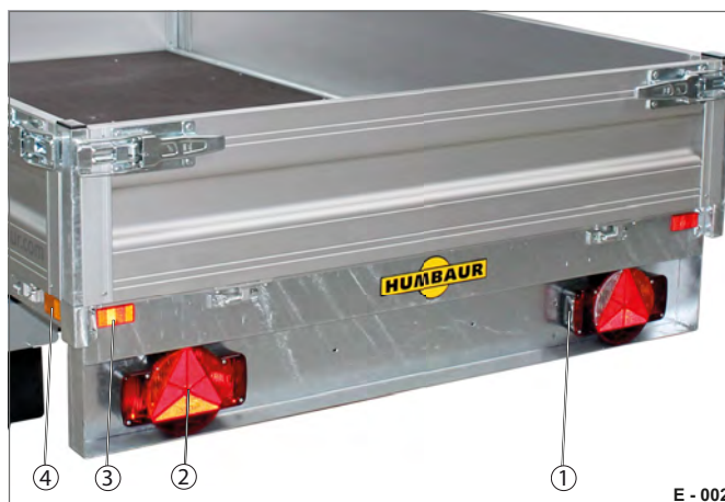
Fig. 2 Lights at the rear
