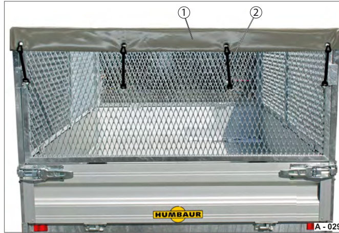
Fig. 44 Example: Flat cover with steel mesh extension
