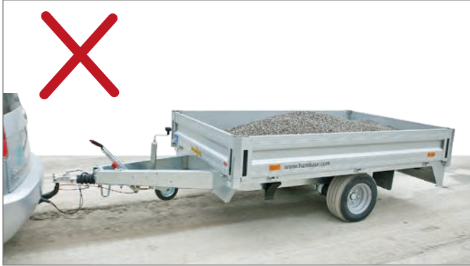
Loose loads not secured
