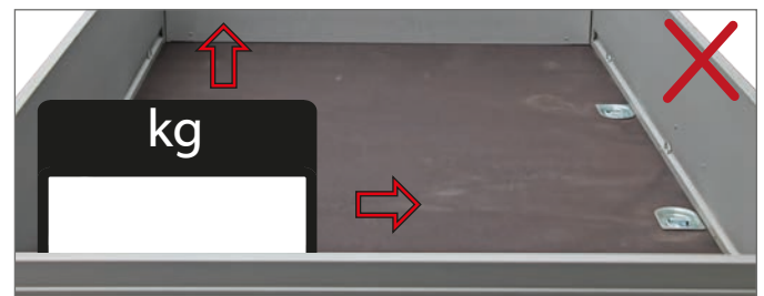
Load incorrectly distributed
