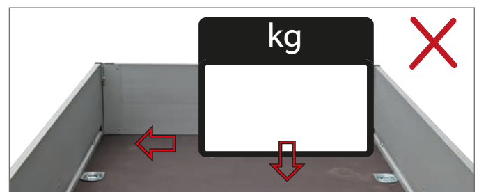
Load incorrectly distributed
